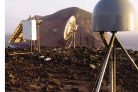
SCIGN stations receive radio signals from GPS satellites overhead...
