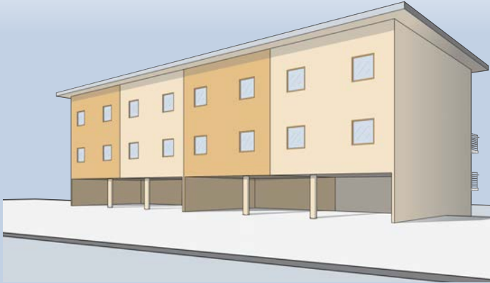
Open structure for parking access lacks first story strength creating a weak story condition.
